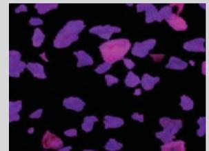
InGaAs Technology provides much better separation of good product from same colour foreign material, in comparison to the visible camera.
