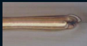
High frequency DC pulse weld
