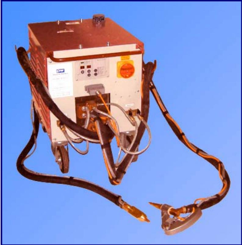
The PP6 weld gun is fully water-cooled and has spring controlled switching, which ensures consistent weld force in all positions. Watercooling is from the self contained system within the console, which has fan assisted cooling through a heat exchanger to ensure electrode tip temperature is minimised.
